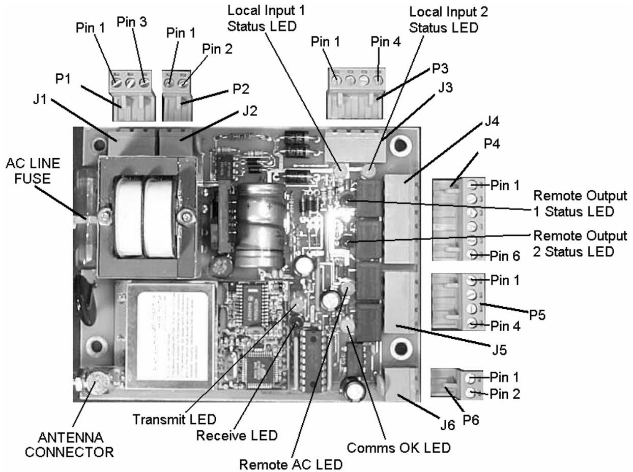
This diagram identifies components, connectors and LED's on the RFSkada board assembly. Refer to the following chart and detailed notes for an explanation of items identified.
